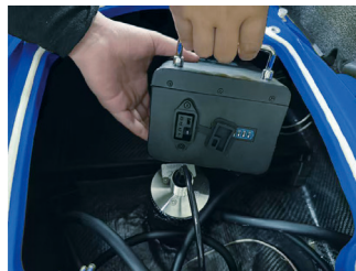
Figure 2.4.1.1 Battery Installation of Tboat10
