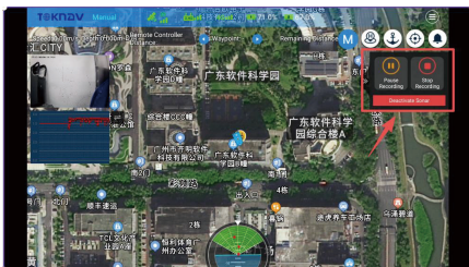
Figure 6.5.8 Pause and Stop Water Depth Data Recording
