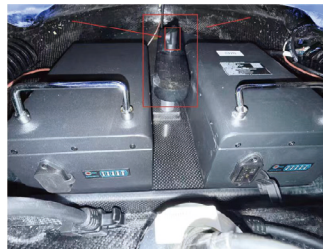
Figure 2.4.1.3 Tboat10 Battery Secured and Power Cable Connected
