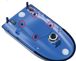
Figure 2.4.1.5 Tboat10 Hatch Cover Installation
