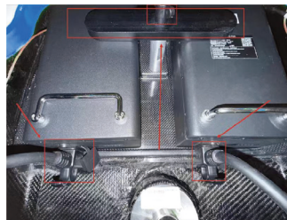
Figure 2.4.1.2 Tboat10 Battery Installed in Place
